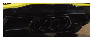
The exhaust manifolds have changed, too, for obvious and not so obvious reasons. "Tri-Y tubular exhaust headers reduce restriction and turn upward to route exhaust over the rear axle," Thompkins said. The muffler was reworked to reduce restriction and improve sound quality, while rear-fascia-mounted bezels are shaped to help reflect some of the sound back to the driver.
