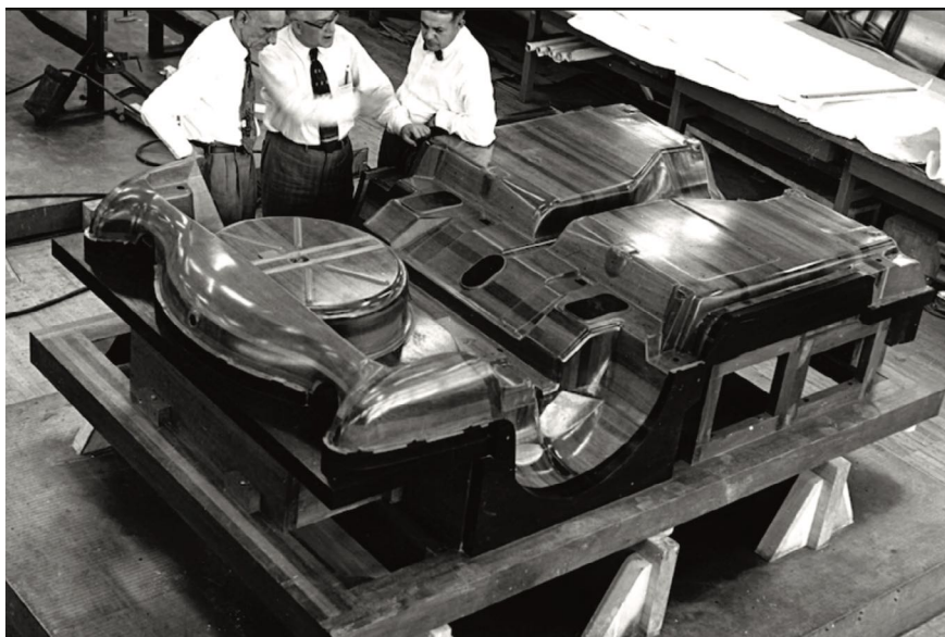
Mahogany Works of Art Are Body Dies for the 1953 Corvettes
